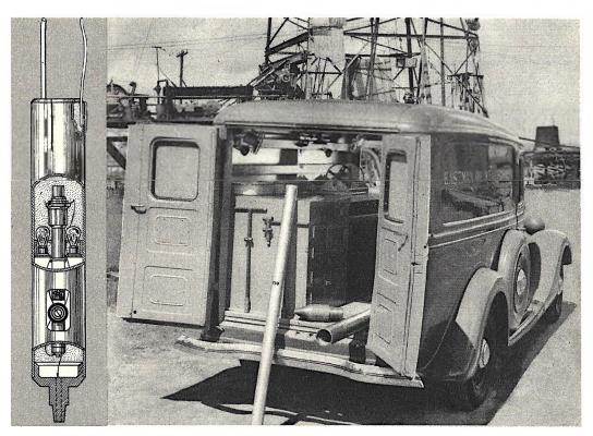
Left—Sectional view of the sub-surface camera showing arrangement of the timing device, flash bulbs and lens (pointing downward). Above—The specially fitted survey truck. Note the facilities for developing and enlarging the sub-surface photographs.
