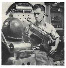
DEVELOPED by Ive Vestrem, of Milwaukee, Wis., for deep-sea divers working in shark-infested waters, a new high-powered pneumatic rifle shoots harpoons under water. The firing chamber pressure is 2,000 pounds.
