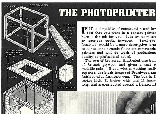
F IT is simplicity of construction and low cost that you want in a contact printer, here is the job for you. It is by no means an amateur outfit, however. "Semi-professional" would be a more descriptive term, as it has appointments found on commercial printers and will do work of professional quality at professional speed.
