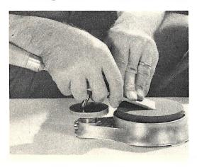
R EQUIRING no special skill, a new automatic oilstone device enables the operator to rapidly produce perfect cutting edges and bevels on hand tools such as chisels and carpenters' planes. The device consists of an aluminum base, one end of which houses a two-sided oilstone, and a smooth steel-topped table on which rests a bronze holder that holds the tool at the desired angle as it passes over the oilstone.
