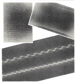
Above are samples of work done with a paint spray gun. A piece of acreen wire may be used to give many novel effects. By holding the wire securely against the work, and with the spray gun pointed directly at it, a clean cut pattern of the wire will result. If the wire is lifted slightly, a different pattern will be obtained, very unusual in appearance.
