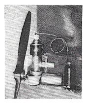
Powerful enough to fly an 8-foot model airplane, this  $4\frac{1}{2}$ -inch "gas" engine was built by Carl Johnk.
