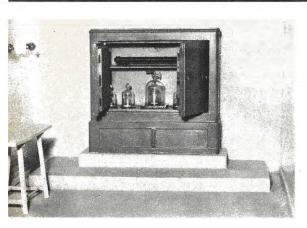
Below is shown an extremely delicate balance which can check a one kilogram weight to within .01 milligram. This balance is kept at the Pavillon de Breteuil, Sevres, France, in an airtight steel vault of constant temperature. In this vault, carefully guarded, are kept the standard meter and kilogram.
