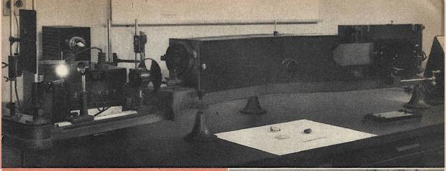
spectrograph breaks up light into its compo-wave lengths or colors for analysis. It re-markings on writing pads and other impressions.
