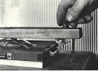
Right: When the lever is lowered, the long screw pushes down the plunger of the exposure switch. The latch may be used to lock the platen for long exposures or local control. Below: The platen lever parily raised to show pressure springs, chain, and coil spring. See construction details above.
