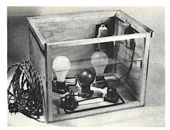
The printer with one side removed, show ing arrangement of lamps and glass for diffusing tissue.
