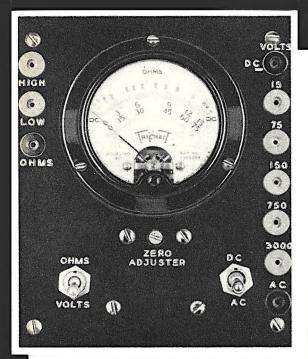
A GOOD multimeter is undeniably the most useful of all test instruments for anyone who works with electrical apparatus. Yet the high cost of the more elaborate commercial instruments has prevented many from purchasing such a device. Though the MECHANIX ILLUSTRATED "Testmaster" to be described is inexpensive and simple to build, it has been carefully engineered to give the utmost in ease and accuracy of operation and a wider range of application than many of the
