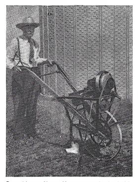
Powered by a washing machine motor geared to its wheel by a sprocket chain, this cultivator was built by Marion Long.
