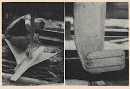
The specially designed anchor (above, left) drops from the bottom of the boat. At the end of the shaft is an anchor chain. The protruding end of the stabilizer is shown at right. It protrudes, through a shaft in engine room, below the keel.
