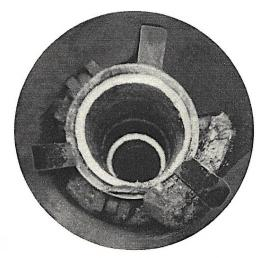
A photograph of the interior of an oil well casing taken by the sub-surface camera at a depth of more than 5,000 feet.
