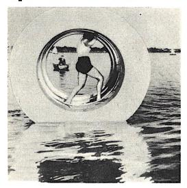
A NOVEL aquatic gyro wheel by means of which he propels himself over the water by rolling over and over has been constructed by H. Schulze, of Hanover, Germany. The wheel is built of wood and light metal.
