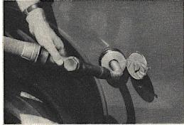
A NEWLY developed theft-proof gas tank cap is fitted with a flexible spout (top) which is installed permanently within the neck of an automobile's regular gas tank, (lower). An internal grill prevents siphoning of gas by thieves and eliminates "blow back" caused by air in the tank at filling time.
