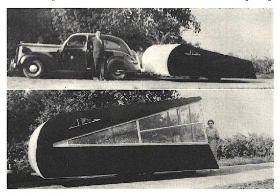
A DUAL-purpose house trailer (lower photo) which features an upper section that can be folded flat when traveling (top), enabling the driver of the tow car to see back over the road by means of his rear view mir-
