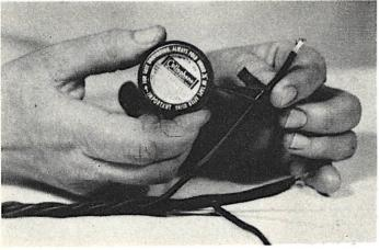
BOVE - Colored tape A wrapped around plug-in coils serves two useful purposes-holding the windings in place and identifying the frequency band of the coil. Each coil should be marked with a different color. Left —Small strips of colored tape can be used to good advantage as code markers for a group of wires, such as a battery or power supply cable. wire should be given a separate color or combination of colors.
