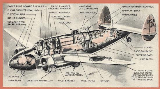
This cut-away perspective drawing shows how the space aboard the world-circling plane was utilized.
