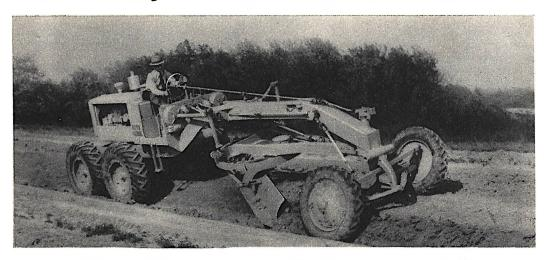
POWERED by a 66-horsepower diesel engine, a newly developed road grading machine features a blade which can be turned completely around, providing a means of
