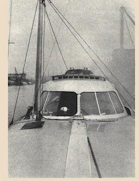
The off-center mast is collapsible. The roof of the pilot house raises 6 inches for ventilation. Note smokestack louvres designed to create upward air currents to carry off engine smoke. All exhausts are through this stack.
