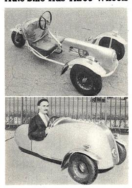
R ESEMBLING a midget auto in appearpearance, but pedaled like a bicycle, a new three-wheeled vehicle has recently been developed. The photos above show the car with and without its sheet metal body.
