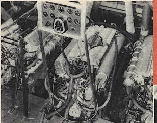
The engine room of the Q.E.D. is all engine. The center one is an 800 hp. diesel. End ones are 600 hp. Capitol engines.
