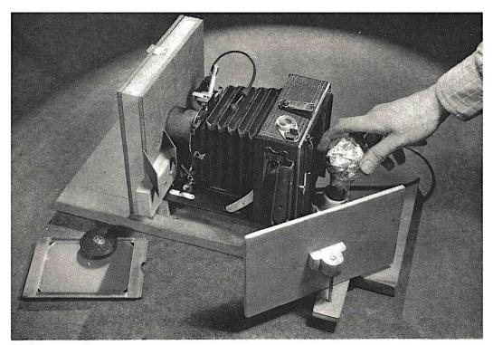
The completed tester from the mirror side. Note that large mirror, whose back is toward the camera, can be adjusted for angle. Back of camera has been removed.
