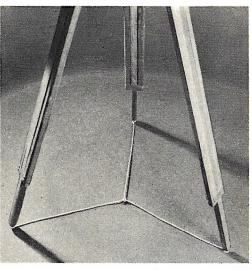
Cut three 15-inch lengths of galvanized wire and bend the ends into loops with one end of each fastened together. They can then be placed on the floor with the tripod legs resting in the outside loops, preventing them from slipping on any smooth surface. This simple device will do much to prevent accidental damage to a camera by having the tripod slip on a smooth floor. Also, the tripod can be moved easily over the floor with legs remaining in their respective positious.
